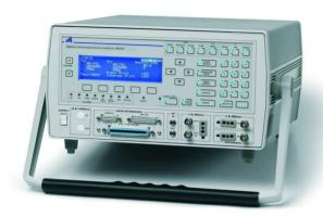
Desktop and rack-mountable digital testers for a wide range of PCM and data measurement applications up to 8 Mbit/s
